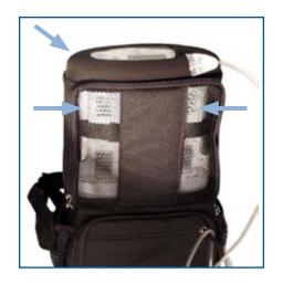
5. Verify vents are not blocked. There is a cut out on the top of the backpack for connection to external power.
