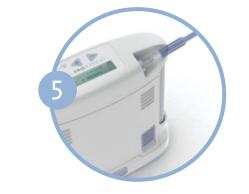
Connect the nasal cannula tubing into the metal nozzle on your Inogen One G3. Oxygen will only be delivered while you are breathing through the nasal cannula connected to the device.
