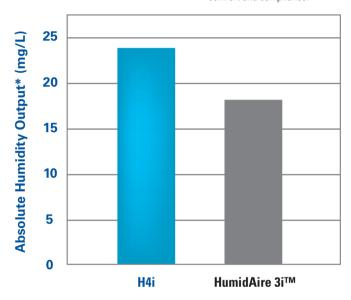
The H4i is specifically designed to produce greater humidification outputs to support the higher pressures delivered during bilevel therapy.
