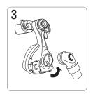
Remove the elbow assembly from the mask frame.
