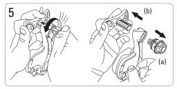
Note the position on the dial for the next time you use the mask. Unscrew and remove the dial (a) then pull the forehead support (b) out of the mask frame.
