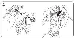
Insert the forehead support (a) into the mask frame and screw (b) the dial clockwise onto the pole. Turn the dial until it clicks (c). Ensure the dial sits flush against the frame.
