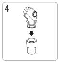
Remove the swivel from the elbow
